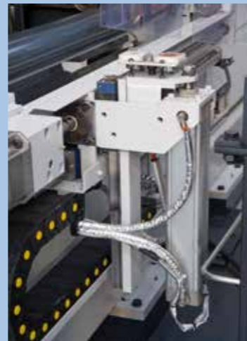
Underside web scribing device
